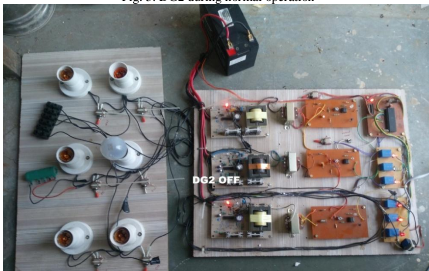
Fig. 4. Short circuit fault occurred on DG2
